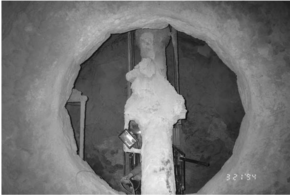
Figure 12.2 Typical cement kiln interior (approximately 8 ft inner diameter—process analyzer sample probe is supported behind left kiln wall).
